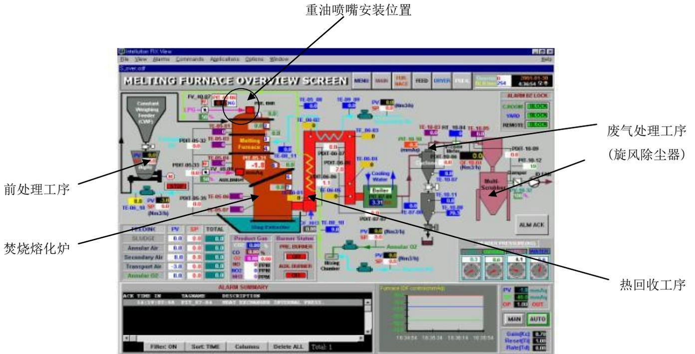
Figure 2. Main control graphic display for melting furnace system.
